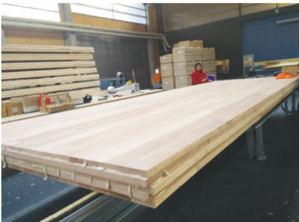
Photo 1: CLT panel from Light Red Meranti.
