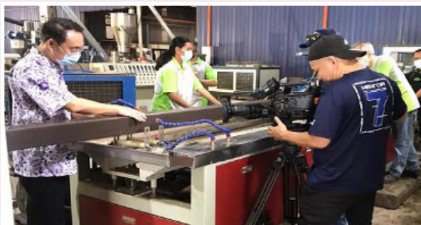
Managing Director of Perceptive Profile Sdn. Bhd. showing the manufacturing process of Metal Reinforce WPC
