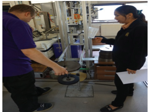
Dr. Loh Yueh Feng, Research Officer of MTIB conducting stability furniture testing with FIRA's technician.
