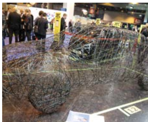
Car skeleton made from carbon fibre.
